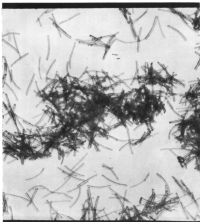
FIG. 1. Suspension of 0.5 mm long sections of natural wool fibers in aqueous buffer solution, pH 4.8, 0.01 M acetic acid + 0.01 M sodium acetate. Flocculated suspension.
